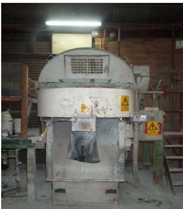
Fig 13: PRECAST Shape Mixer
